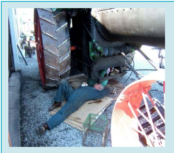
William Bussler and Jerry Delong inspect a boiler firebox of a historic steam tractor.
